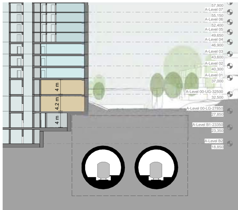
Section through industrial uses
